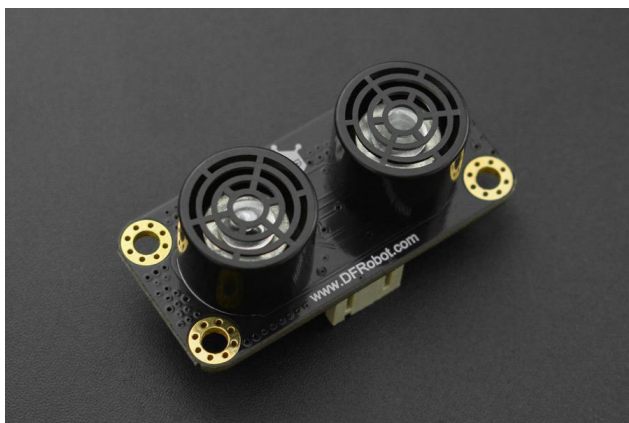
Figure 7: SN0388 Ultrasonic Sensor
