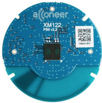
Figure 6: XM122 Acconeer Sensor Module
